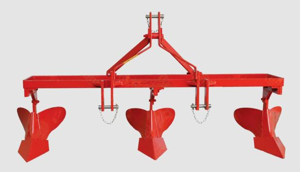
The primary soil tillage machine, **Ridger** is mounted and trailed from tractor's hydraulic lifting unit and universal three-point linkage system. Therefore, transportation to the field can be easily done. Used for making ridges for planting tobacco, potato and other vegetables. The ridger is fully adjustable for giving different accurate row widths. To obtain the correct ridge profile and retain soil flow, the high-grade mould boards are adjustable.
